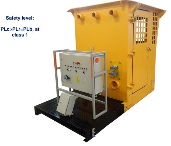
Electrical equipment for the lump breaking device type URB/NPR-6 was designed based on components and certified devices or those possessing declaration of compatibility, equipment is designed for use in the underground mining pits in non-explosive conditions and on the ground.
